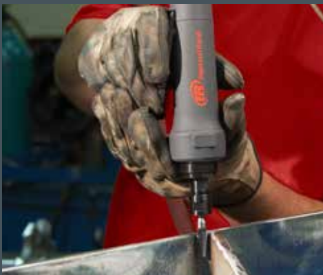
Weld cleaning and smoothing
