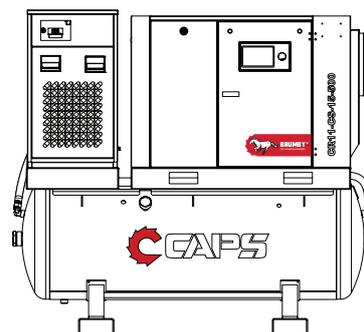
CR11 - CR15 models air dryer is mounted on left side of package
