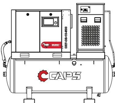
CR5 - CR7 models air dryer is mounted on right side of package
